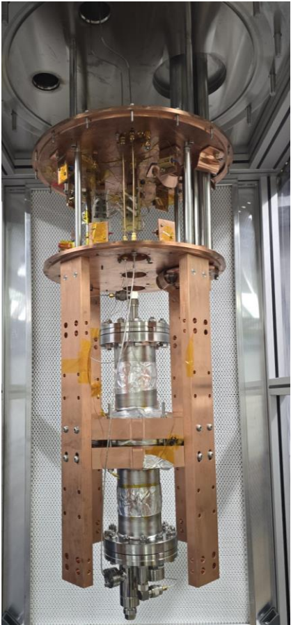
Mounted 1.3 GHz cavity & heat link
