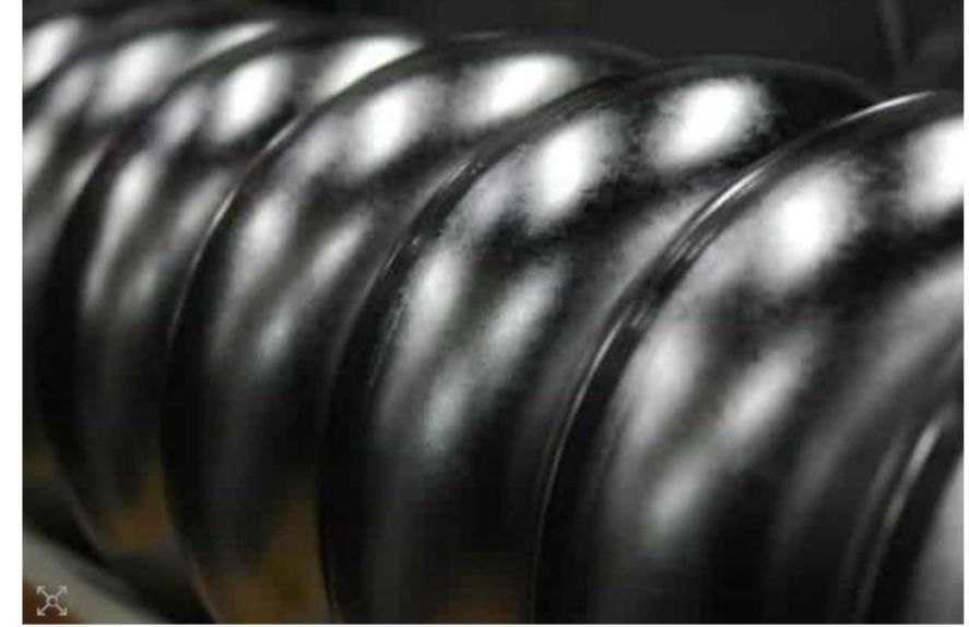
Superconducting cavity for the ILC
