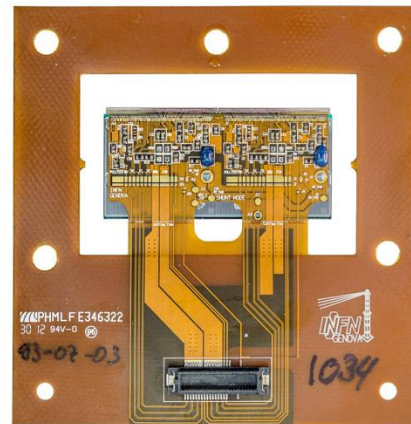
ATLAS IBL – pixel dual- module ( 50 \times 250 \mu\text{m}^2 )
