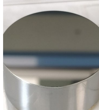
Polished surface (CMP) (Low waviness, low roughness)
