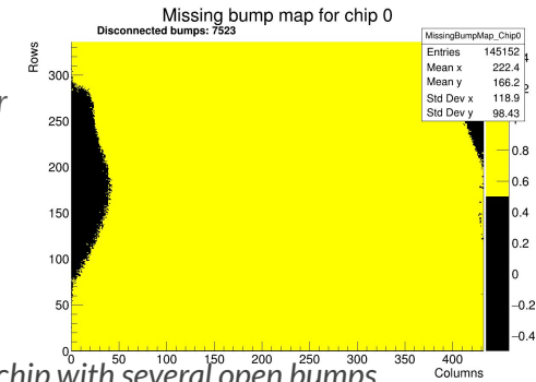
Flip chip with several open bumps, cross-checked also with X-ray measurements
