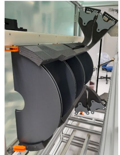
Mock-up of TEPX "octant", Disks + TEPX services in the dedicated box for integration
