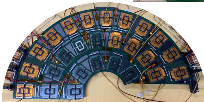
TEPX disk system tests for thermal validation and powering validation
