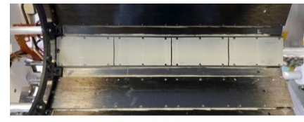
TBPX cradle to host layers, with TIM deposition
