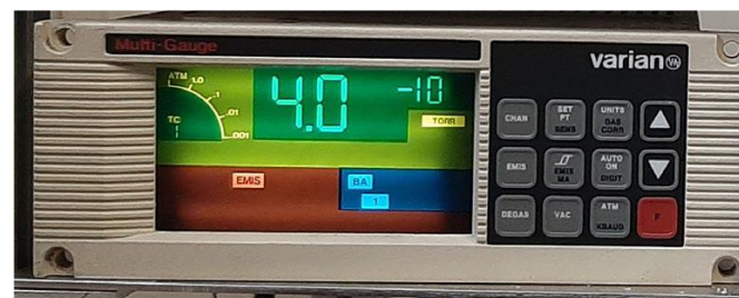
Ultra-High Vacuum Test Setup ( 4.0 \times 10^{-10} Torr \approx 5.33 \times 10^{-10} mbar)
