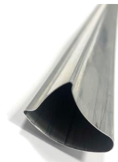
Full Engineering Model #1 (4 aluminium petals, 0.3 mm thick)
