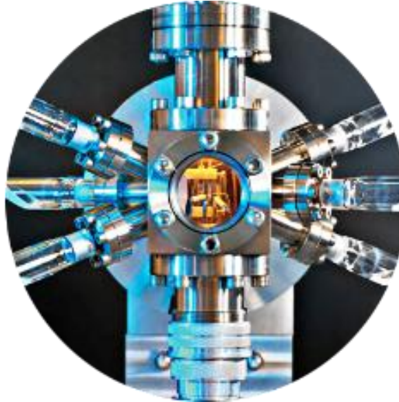
Sr+ ion optical clock
