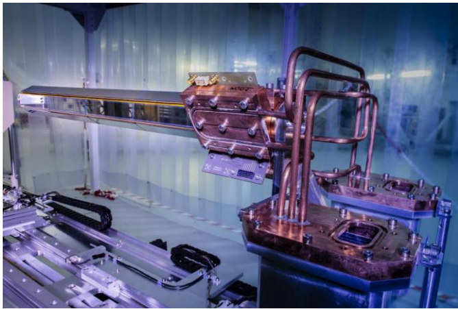
Protons: array of position-sensitive silicon detectors.
