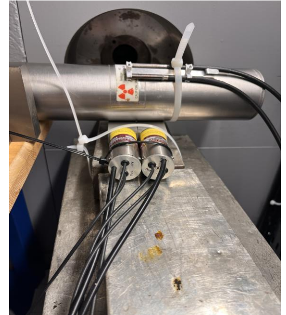
Fission Chambers and Liquid scintillators placed in closed user position
