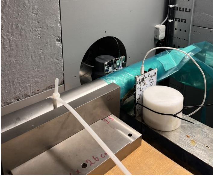
Irradiation of electronic chips at NESSA
