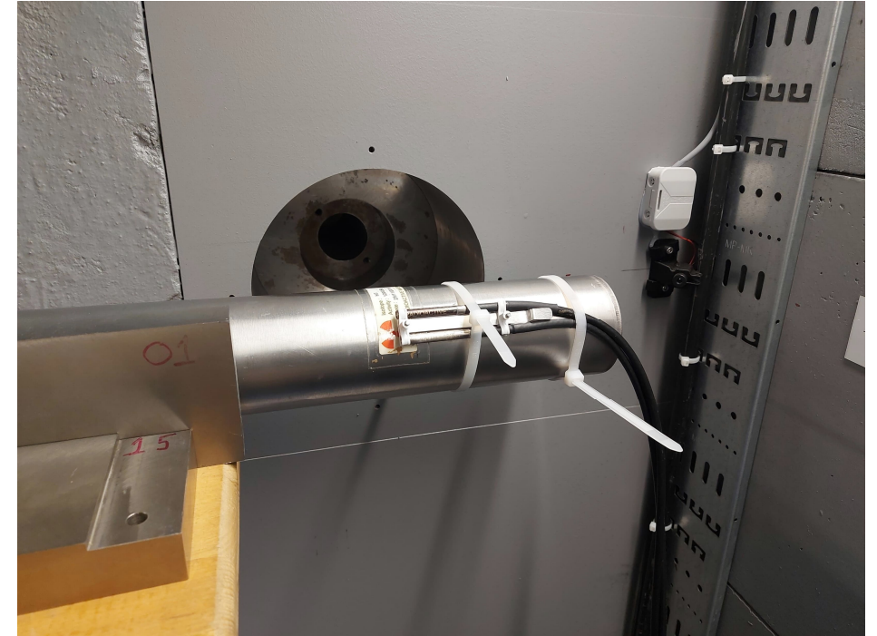
Fission chamber in irradiation positions
