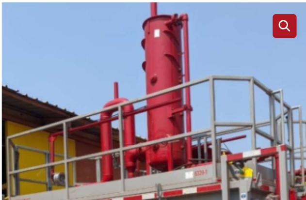
Mud/Gas Separator and Structure
