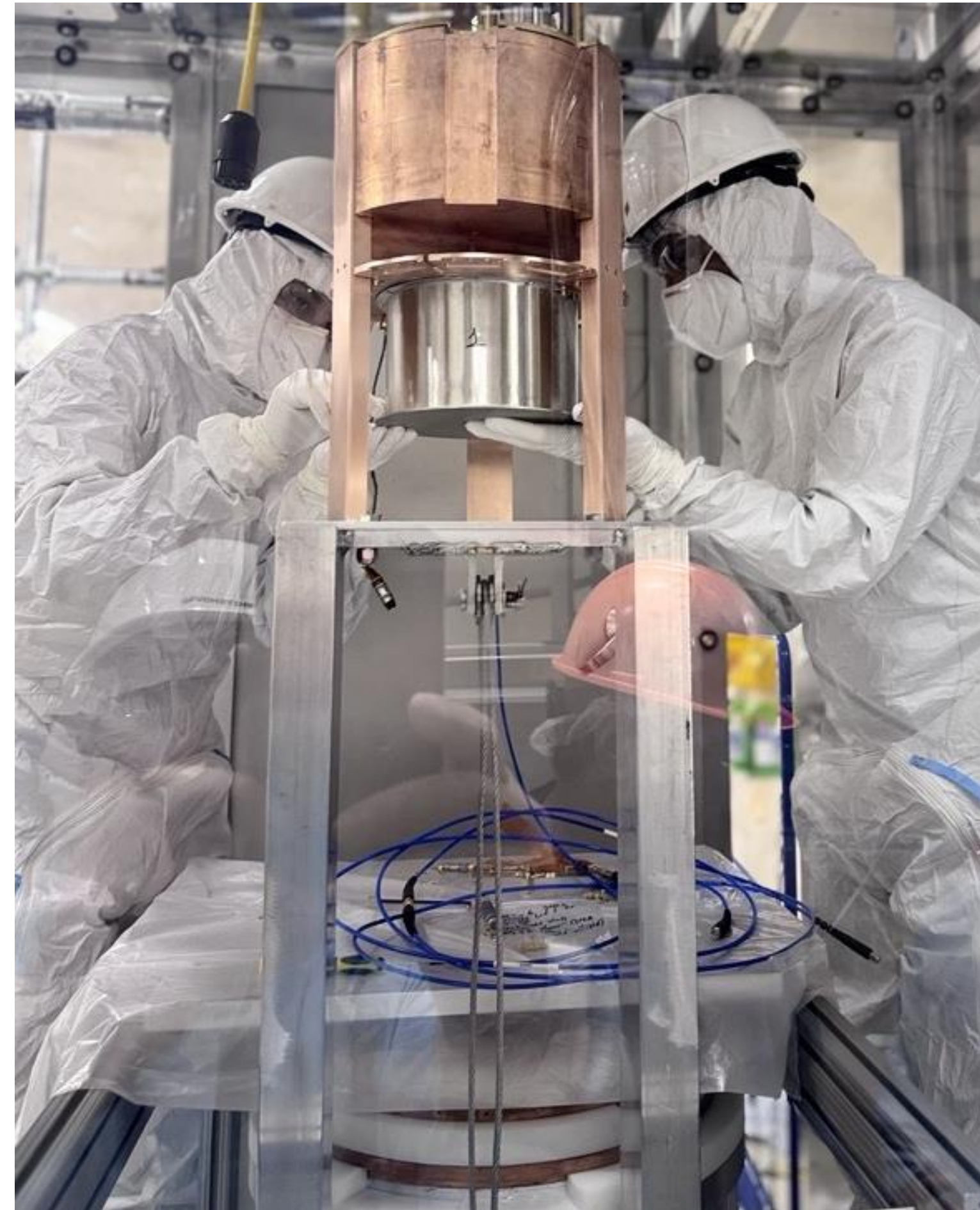
Qubit installation in cleanroom
