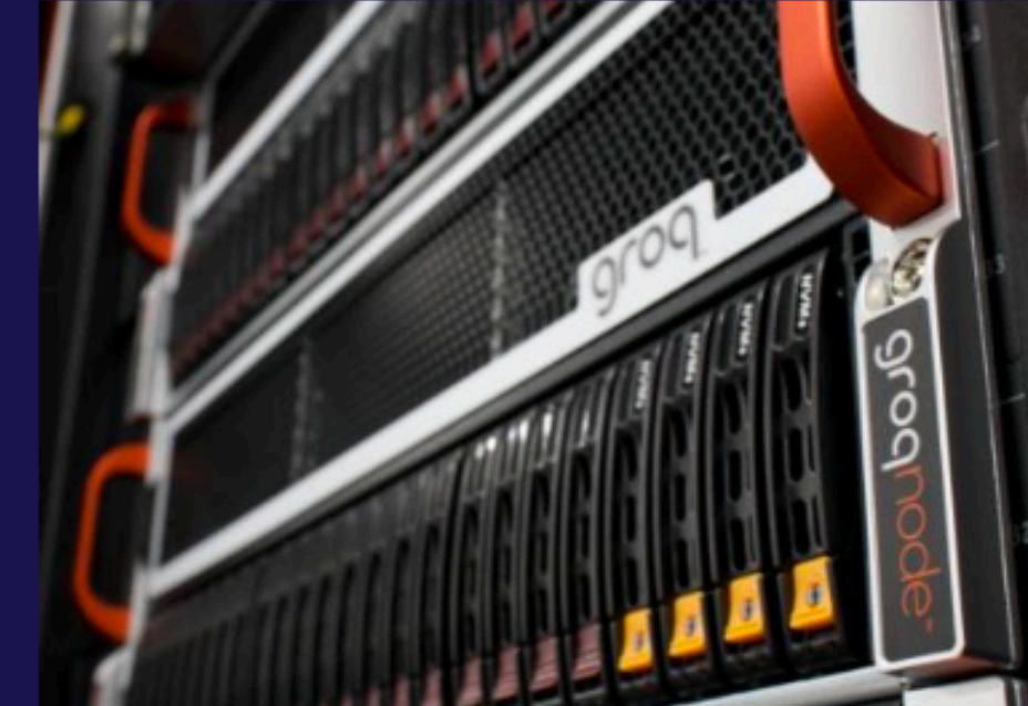
GroqRack 72 accelerators (9 nodes x 8 accelerators per node)
