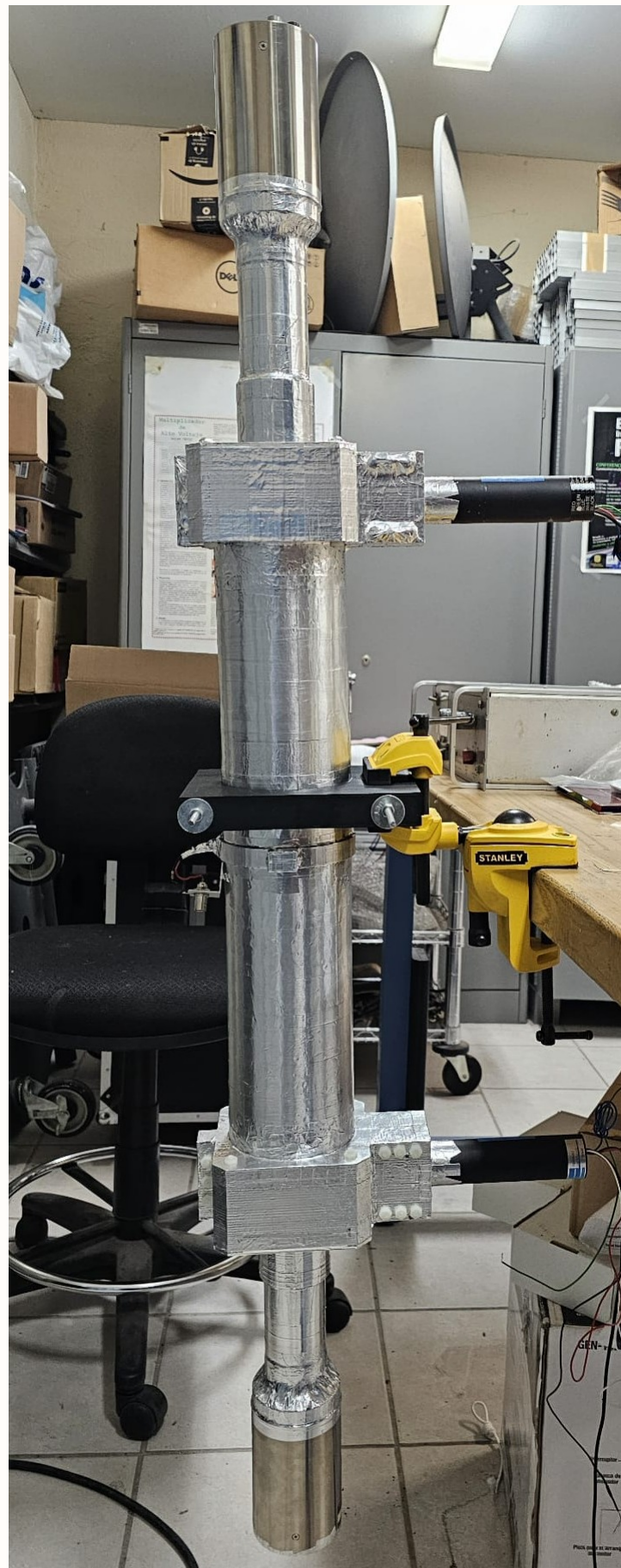
Figure 1: Detector constructed with coupled photomultipliers.
