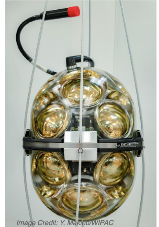
Gen2-DOM PMT segmentation with 4\pi angular coverage in an elongated vessel
