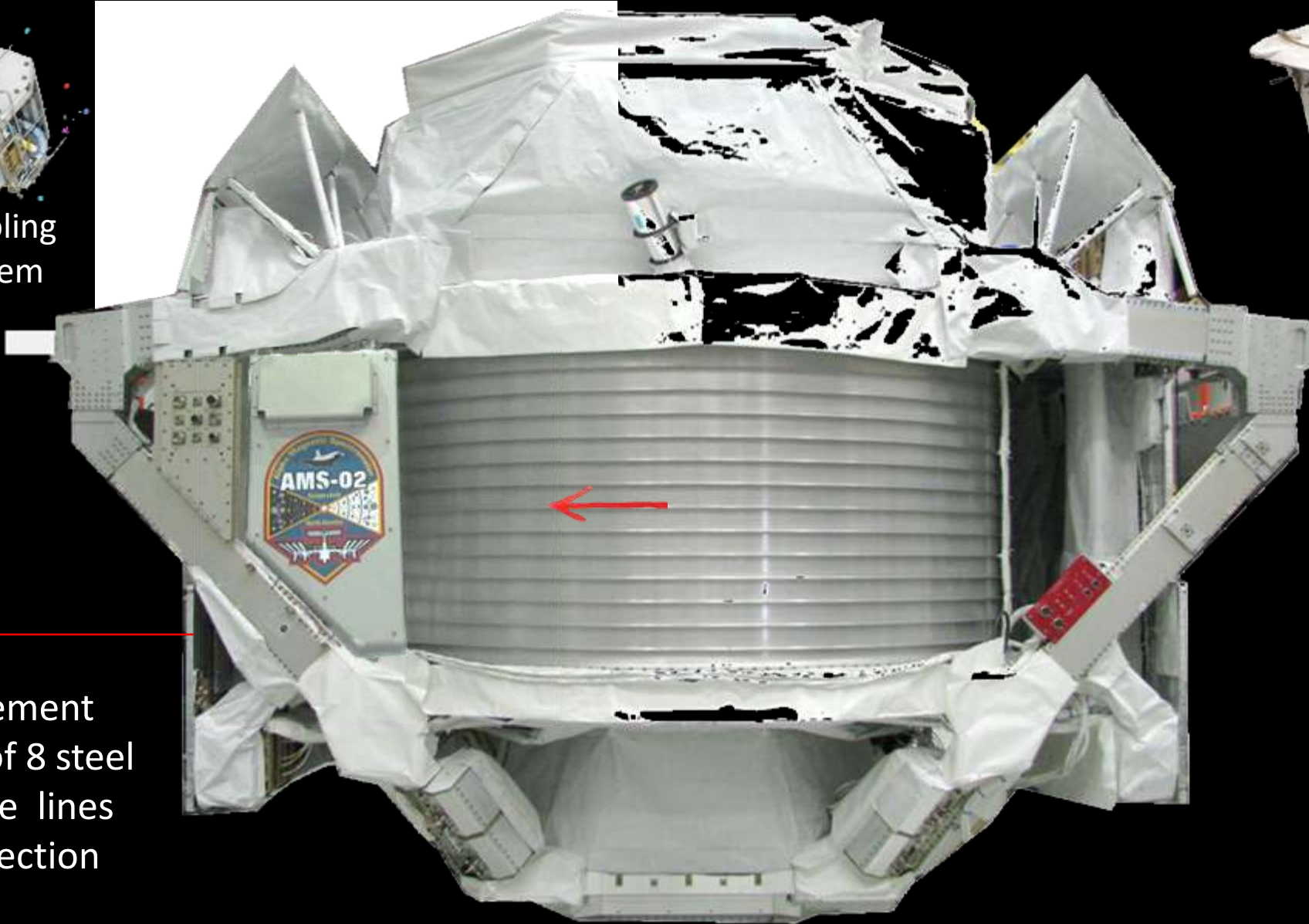
New Pump System was built by AMS for EVA installation
