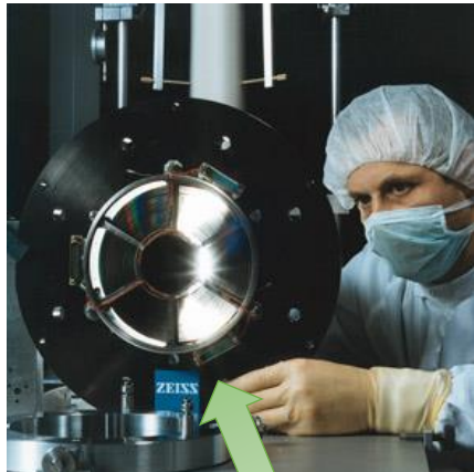
ABRIXAS spare telescope, used in one of the 4 bores of CAST (pioneer use of x-ray optics in axion research)
