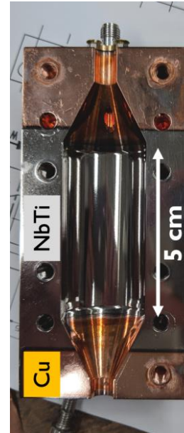
NbTi coated cavity (QUAX experiment)
