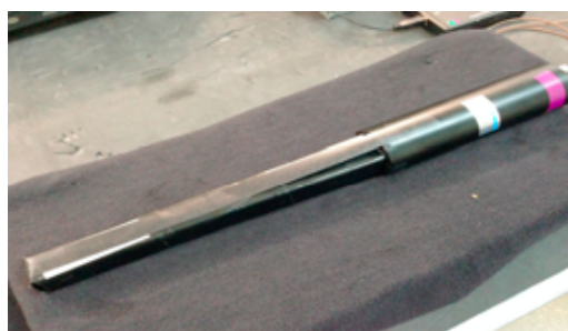
Figure 8: BGO scintillator wrapped and coupled to the PMT.
