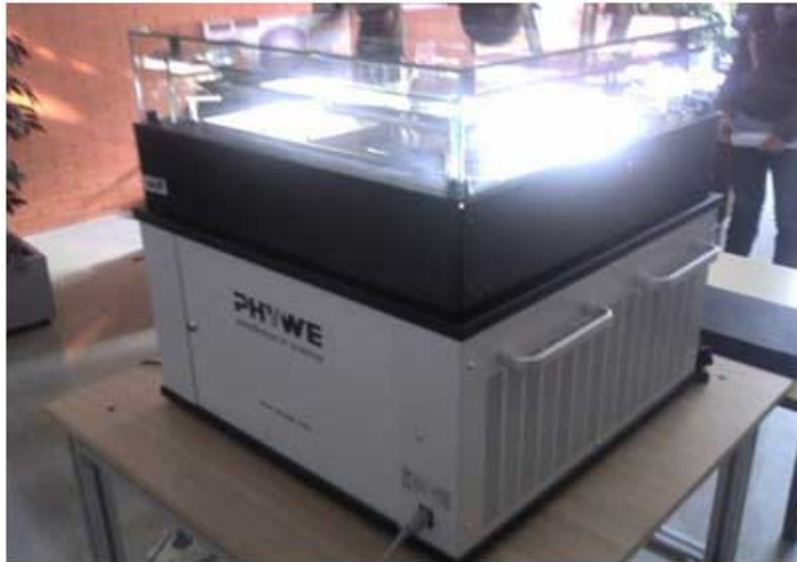
Figure 62: The diffusion cloud chamber used in the practice session.
