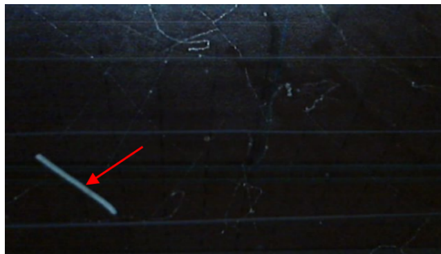
Figure 66: \alpha particle (oblique track) photographed in the IFIC chamber.
