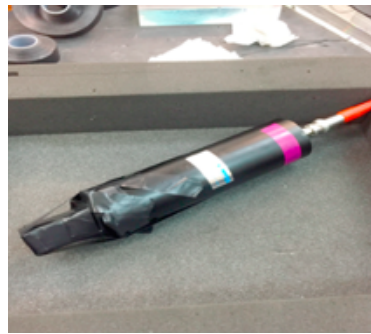
Figure 4: Plastic scintillator wrapped and coupled to the PMT.
