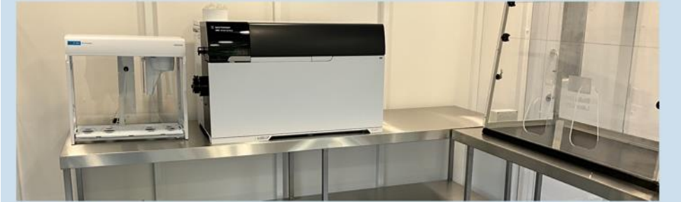
ICP-MS (Surface): Newly installed system for trace element analysis and isotopic ratio measurements.
