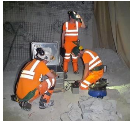
Seismometers and fibre optic acoustic sensors deployed to baseline vibration levels for AION experiment and North Sea regional earthquake monitoring.
