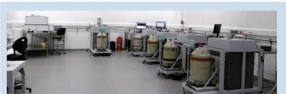
BUGS (UG): A range of HPGe detectors and alpha particle detectors for intrinsic and surface radioactivity measurements.
