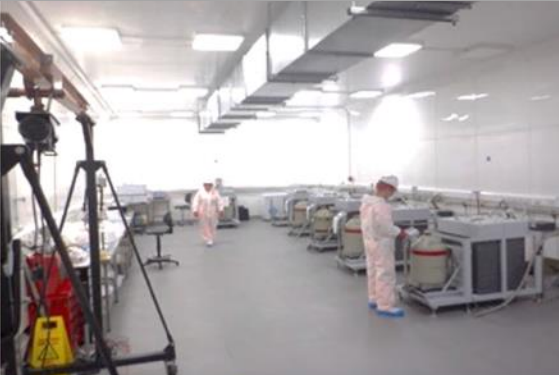
BUGS (UG): A range of HPGe detectors and alpha particle detectors for intrinsic and surface radioactivity measurements.
