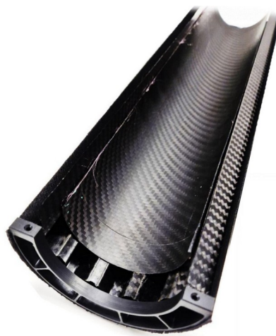
BreadBoard Models: partially representative of the future ITS3, used for cooling studies
