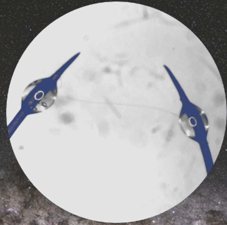
400nm nanowire: NbTi vibrating wire resonators made in Lancaster
