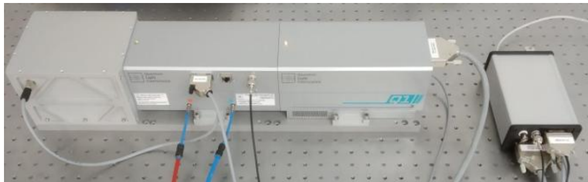
UV laser, 213 nm, 10 Hz pulse rate
