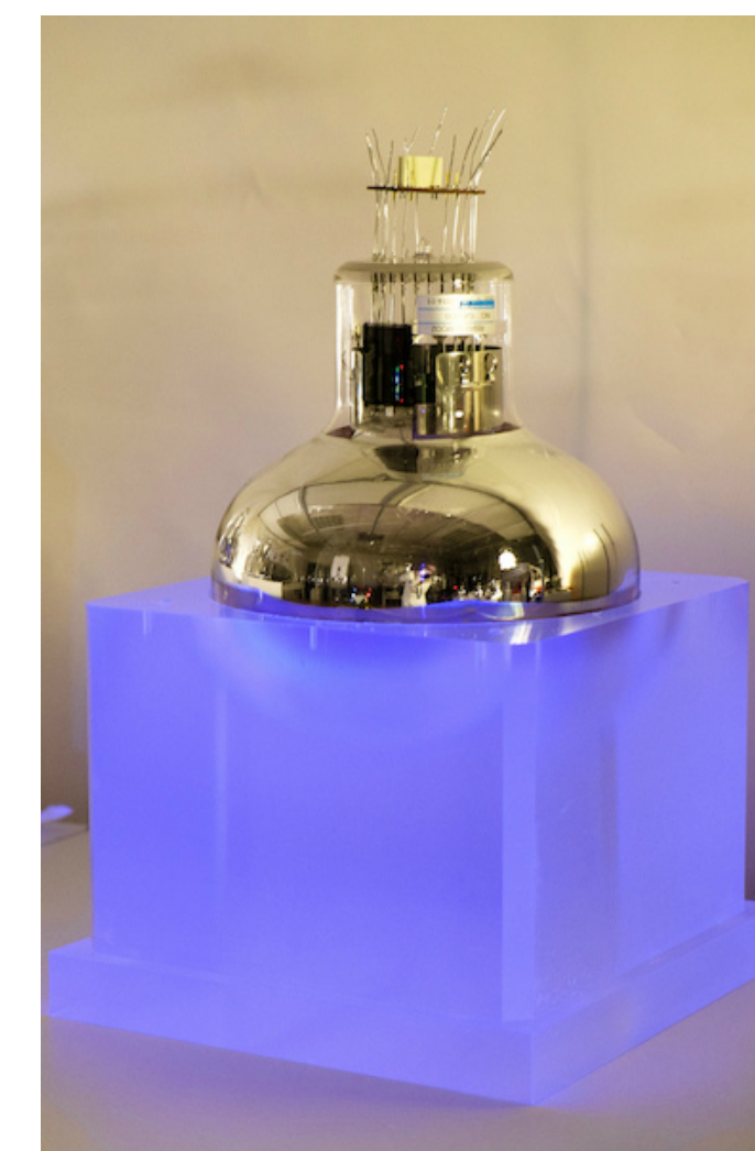
712 optical modules (PMTs with scintillators)
