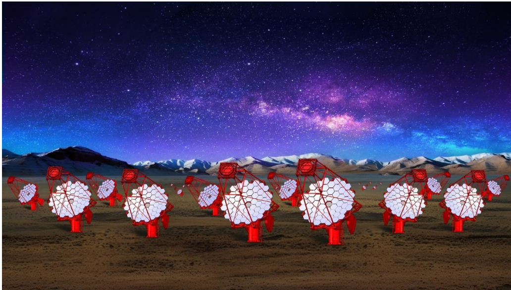
LACT: large array of 32 (+4) IACTs of 6m diameter, f/1.33 at LHAASO site, 4400m a.s.l., largest distance \sim 1.3 km
