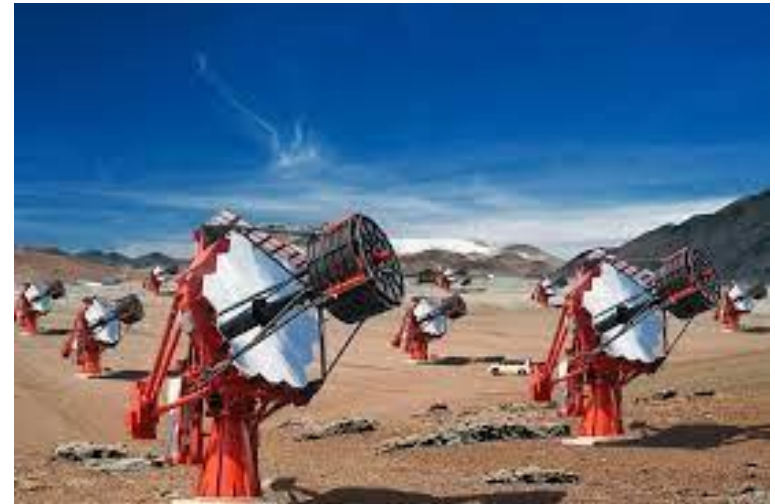
ASTRI mini-array of 9 (+1) telescopes, SCT, double mirror (4.3m & 1.8m) design, on mount Teide on Tenerife on the Canary islands
