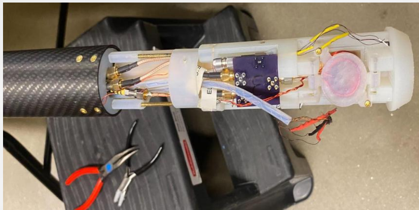
Target cup with cold-board and ssRF and NMR coils
