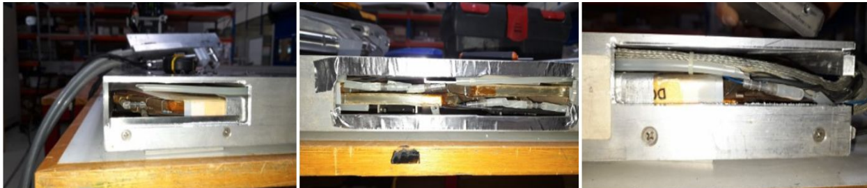
Pilot leak repair in the laboratory with spare chamber
