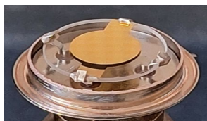
Plano-convex shape (mode confinement)
