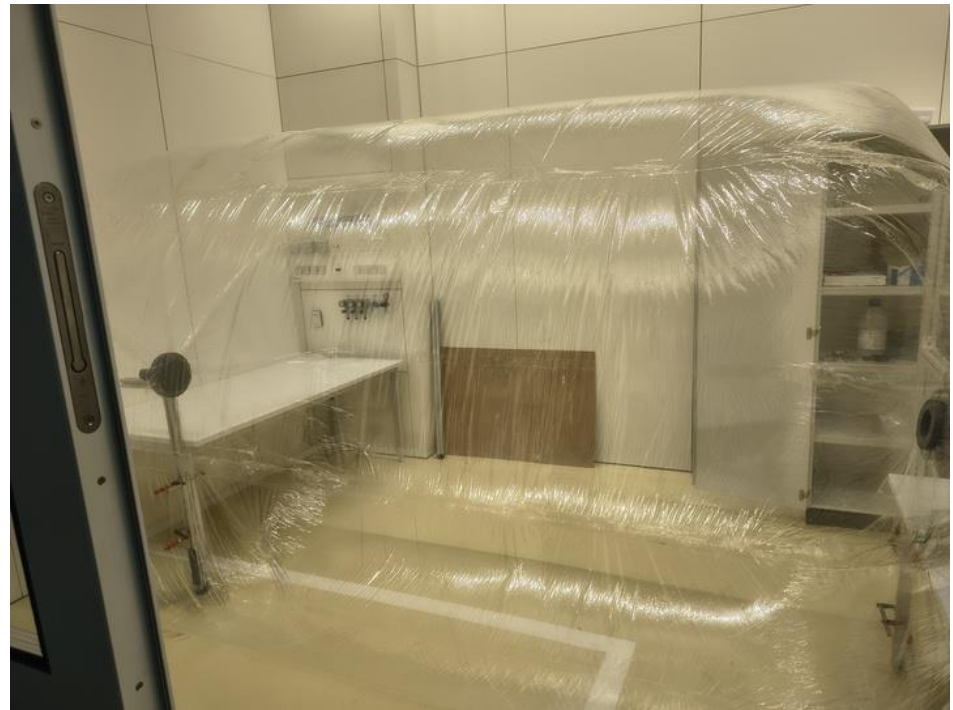
Nylon vessel undergoing pressure test in Mainz
