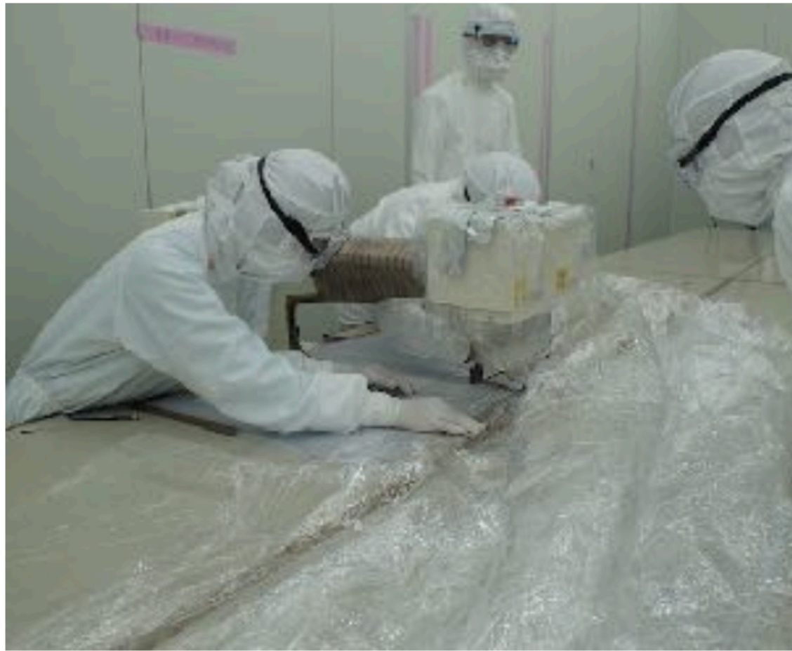
② Seam Welding
