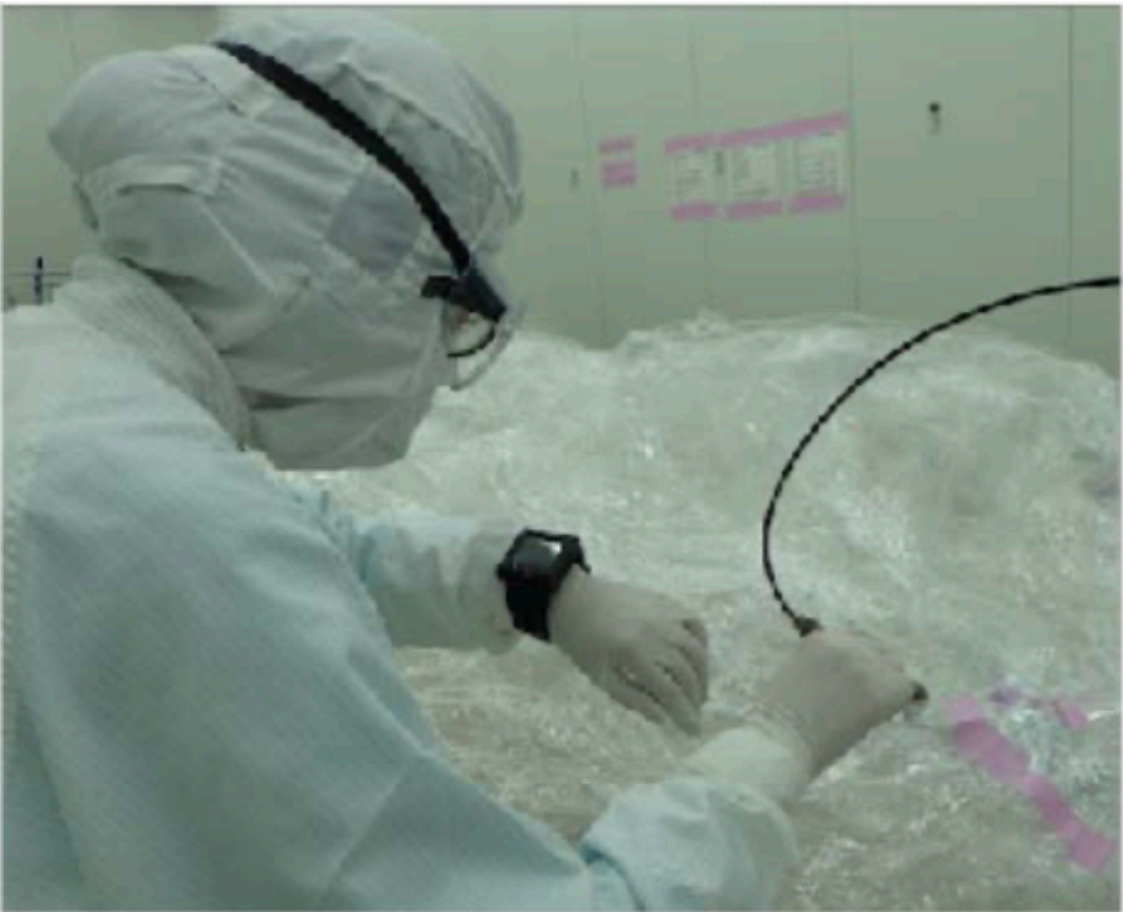
③ He leak test + repairs
