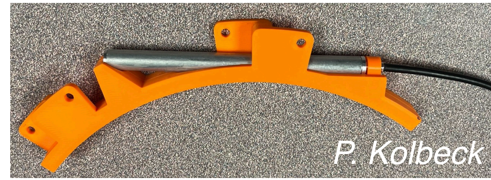
Proton NMR for magnetic field monitoring outside the cryogenic region
