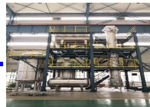
3) Water extraction to remove radioactive impurities
