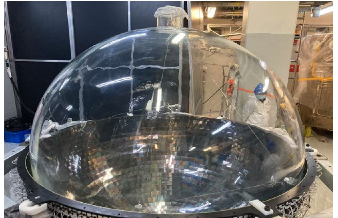
Acrylic sphere assembled (2 cm clearance)
