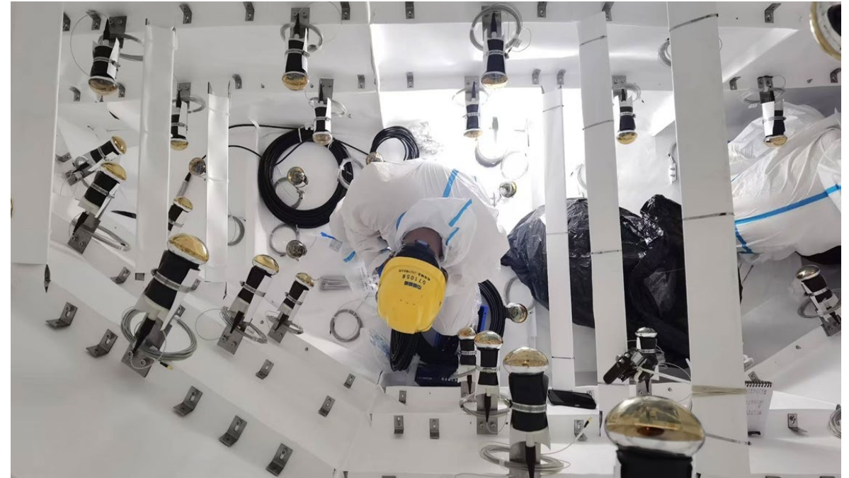
PMT assembly in water tank
