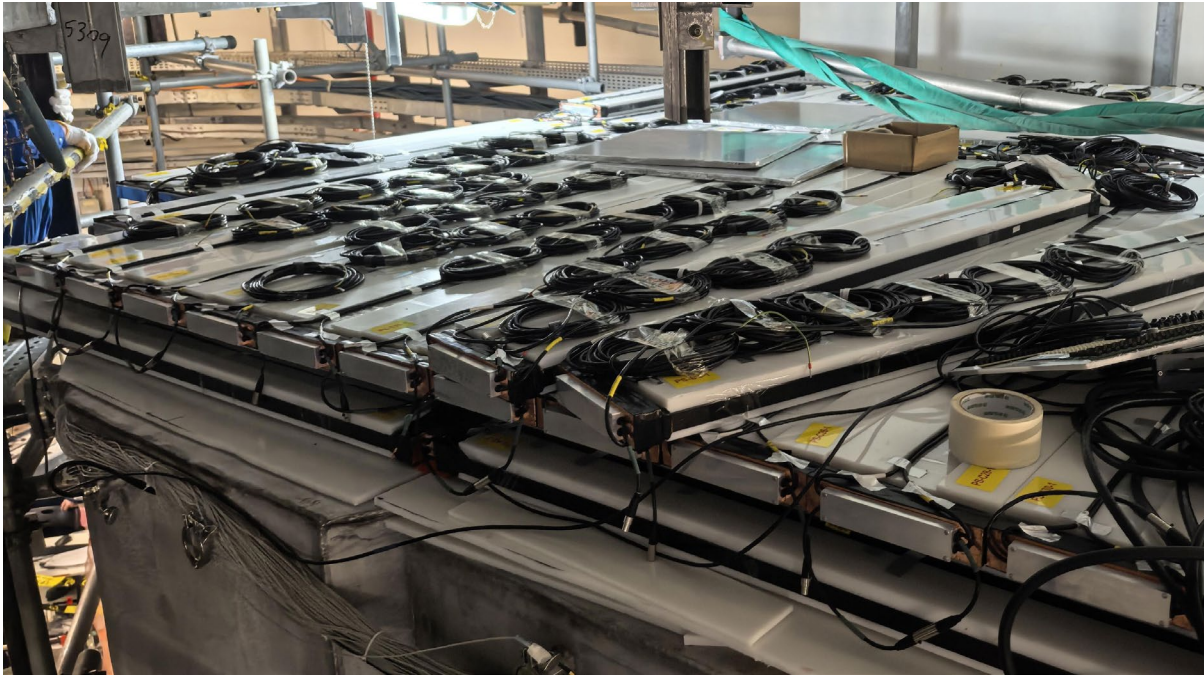
Plastic scintillator strips assembly on top of water tanks
