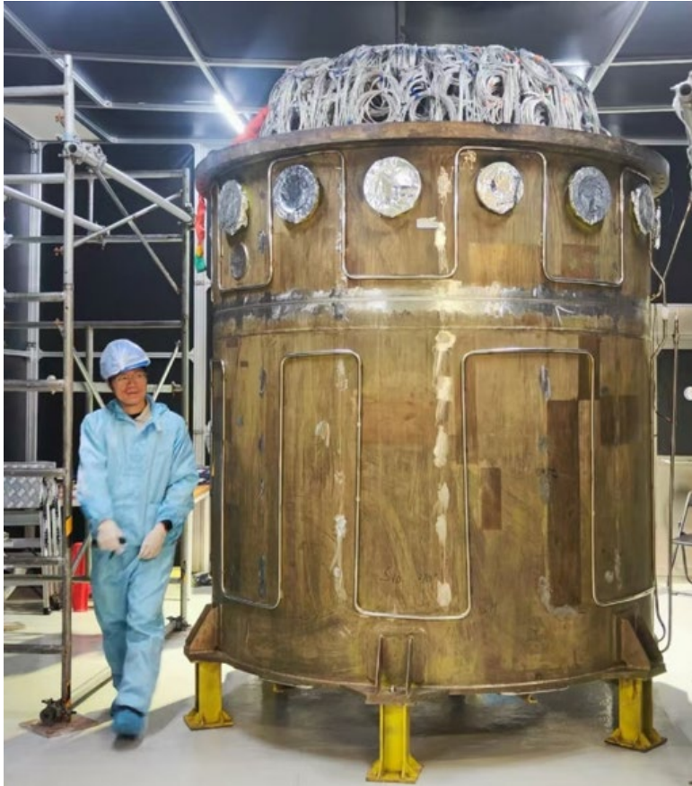
Fully-cabled sphere loaded into buffer tank
