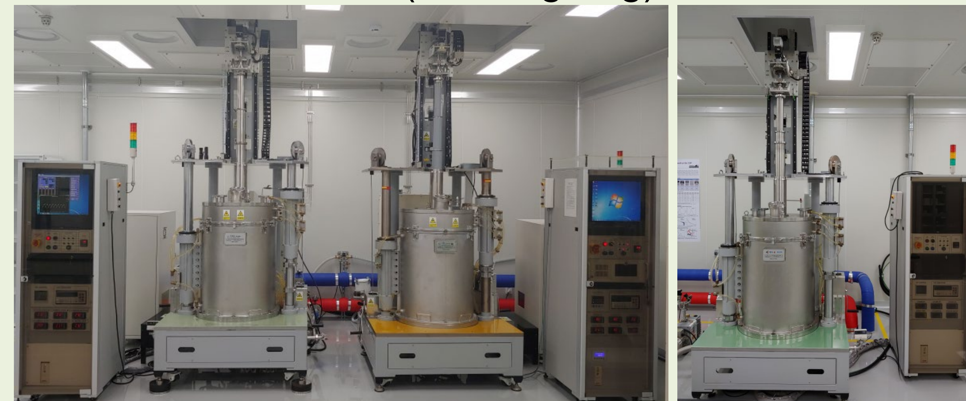
Fig. 1. Photographs of Czochralski growers in the clean room
