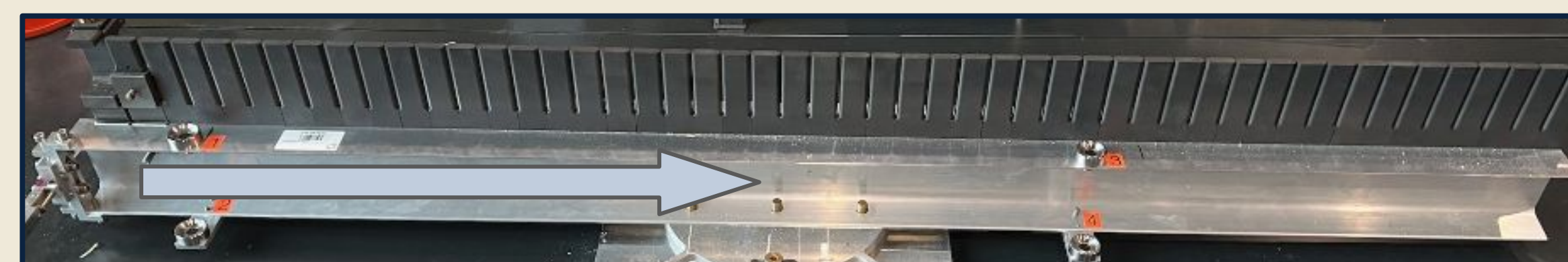
Above: The NuMI Replica Target on a table. Arrow added to show beam direction.
