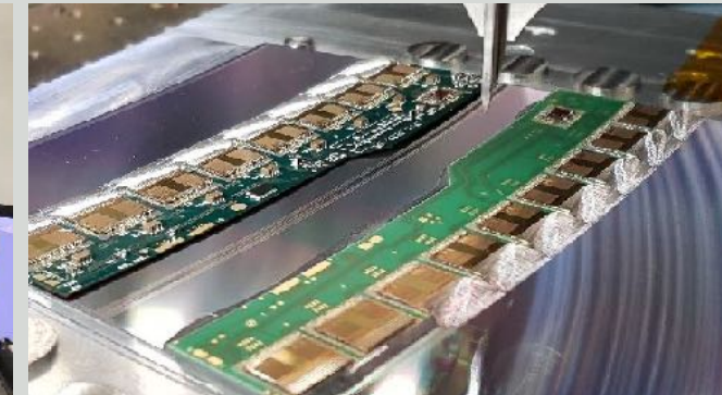
Wirebonding of Hybrid to Sensor
