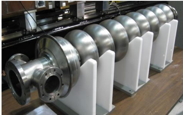
30MV ARIEL SRF 10mA electron linac @ 1.3 GHz first beam 2014
