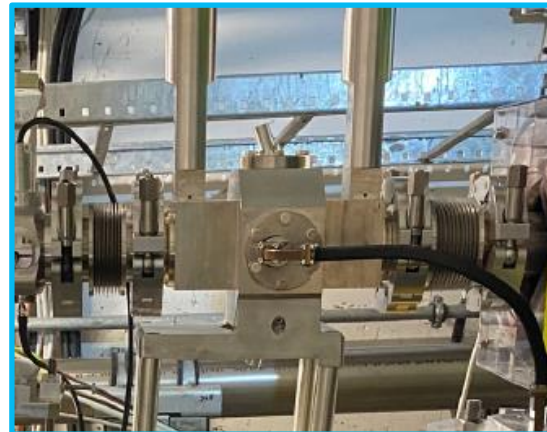
Beam position monitor
