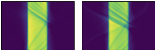
Figure: Sinograms of a slice of an acquisition with only a phantom (left) and phantom and hardware (right).
