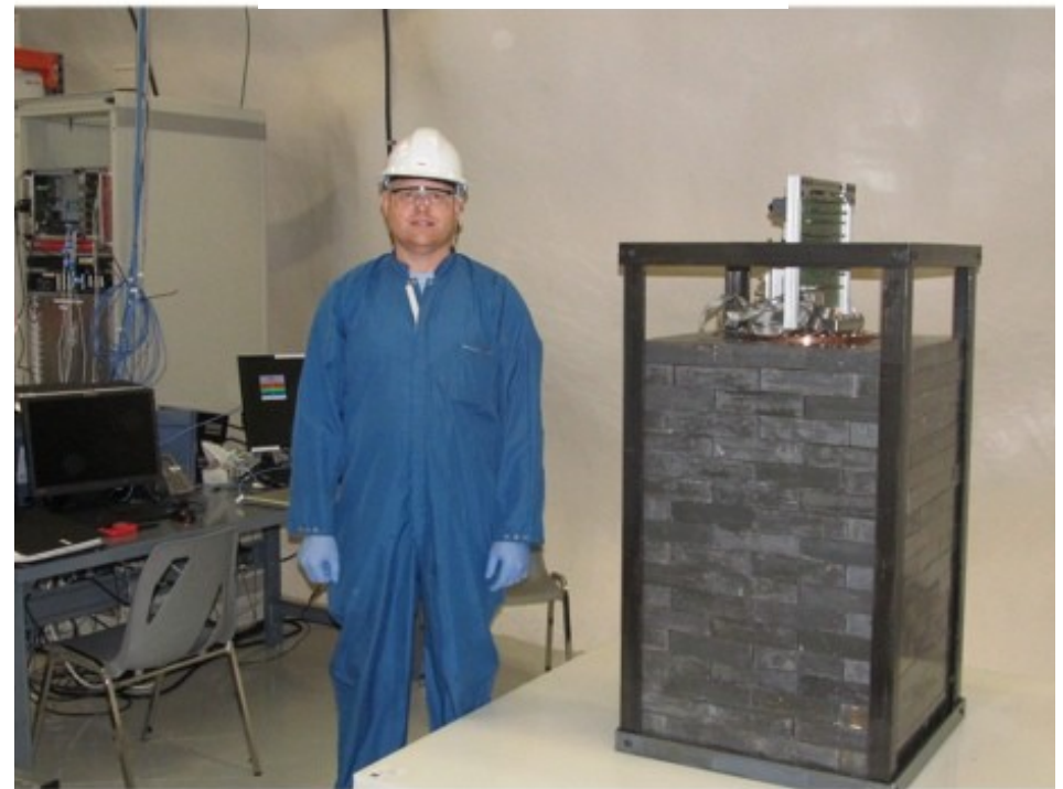
Lead shielding at appropriate thickness
