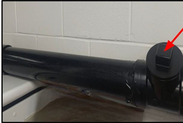
Figure3: Dark box made of ABS Pipe.
