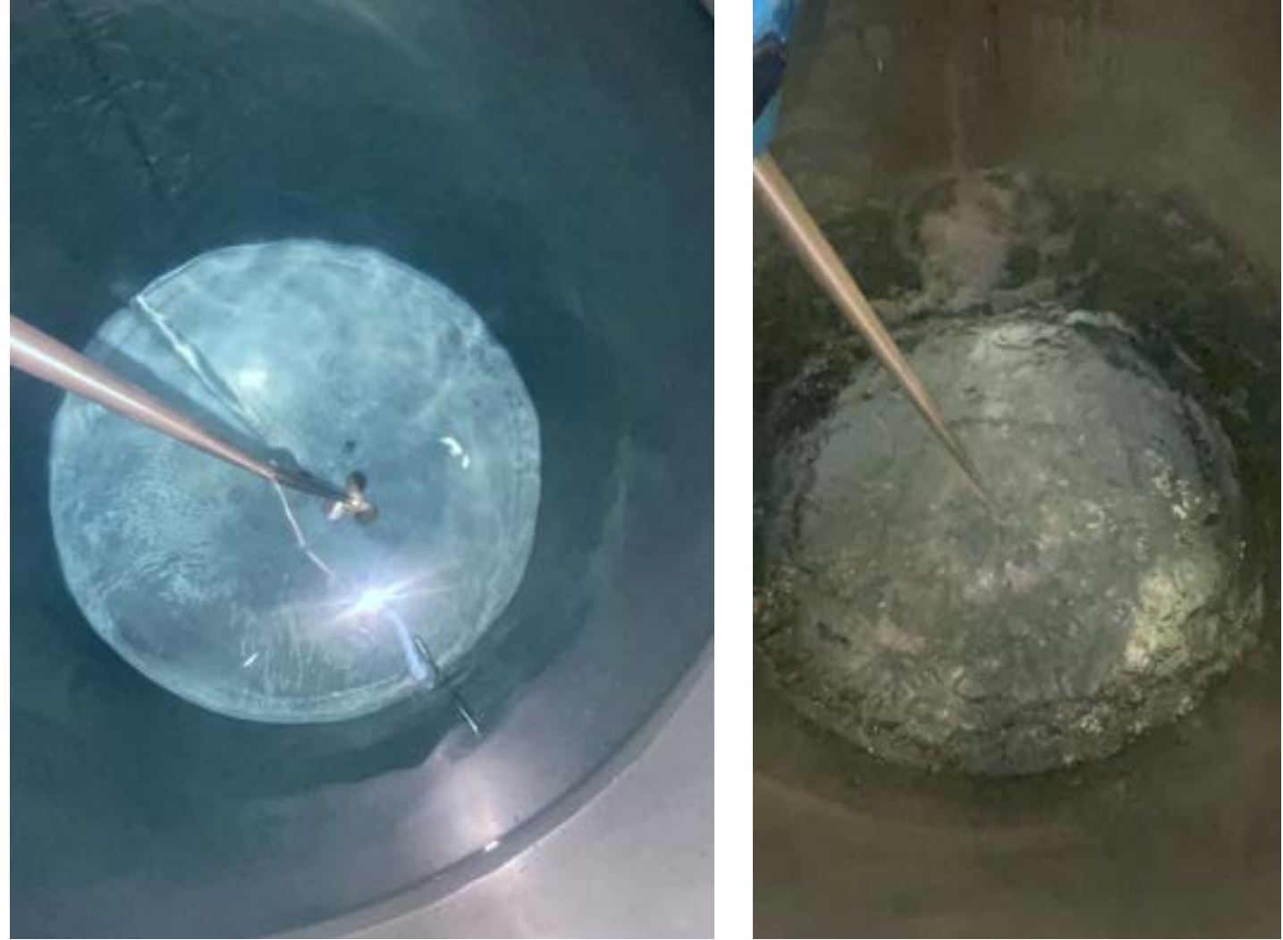
Gd is mixed using motorized mixer in Gd-mixing tank
