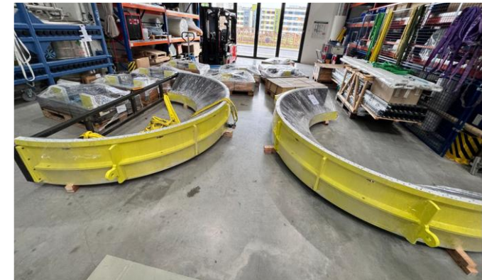
Detector shielding and holding structure
