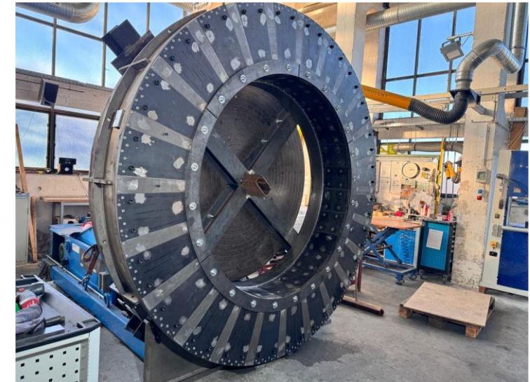
Detector shielding and holding structure
