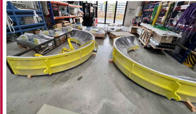
Detector shielding and holding structure
