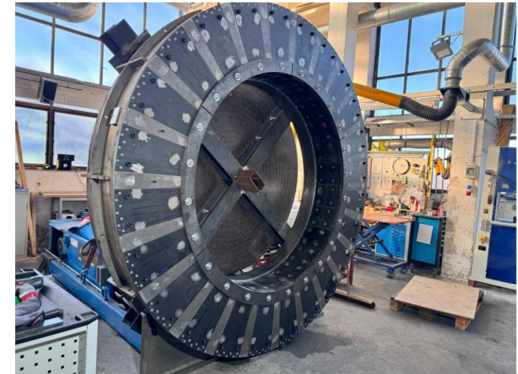
Detector shielding and holding structure
