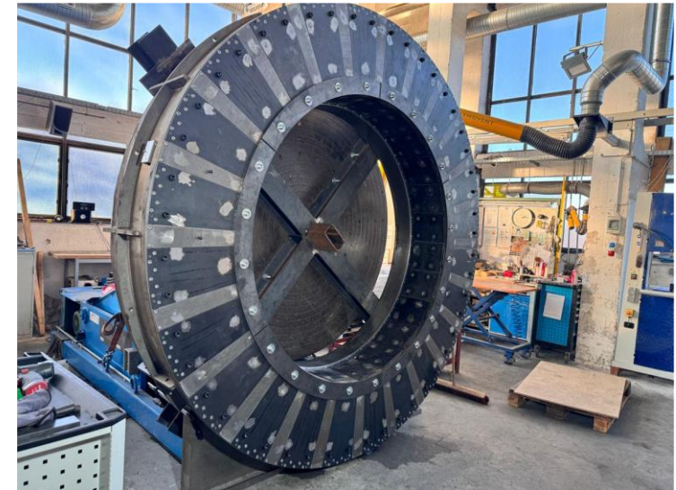
Detector shielding and holding structure
