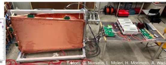
Cosmic ray test of EIL4 triplet with new ATLAS readout system
