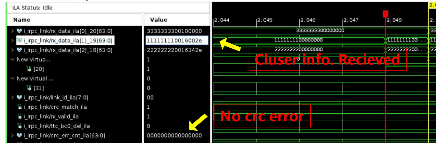
Data receive window from EMTF side
