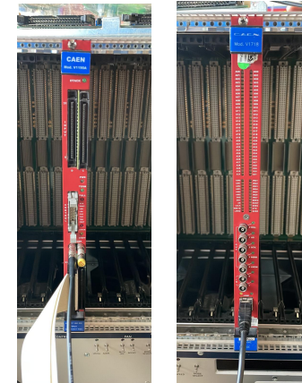
TDC and VME bridge
