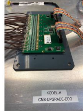
iRPC prototype opened and KODEL electronics
