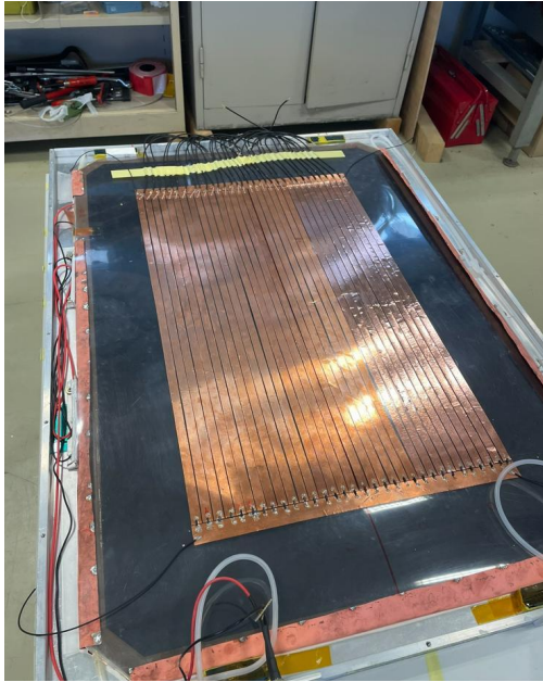
Chamber strip plane with copper tape example
