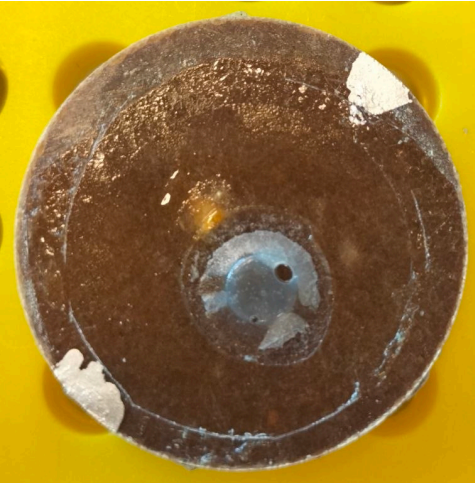
Bakelite sample from HV electrode
