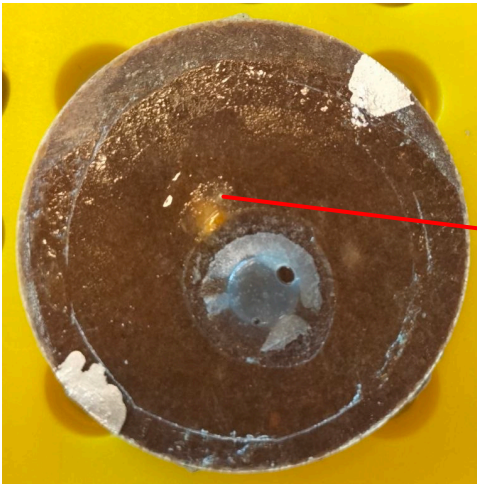
Bakelite sample from HV electrode
