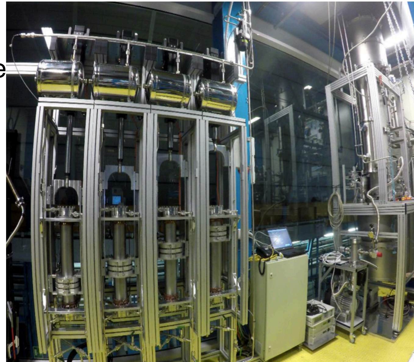
Radon Distillation Column
