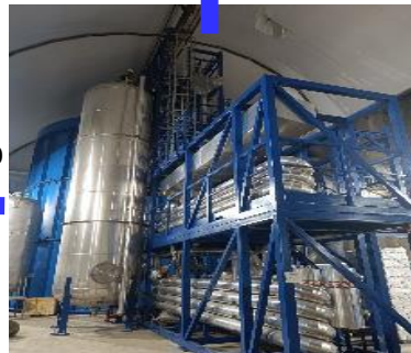
4) Gas stripping to remove Rn and O 2
