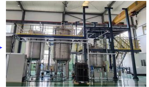
Mixing LAB with PPO and bis-MSB
