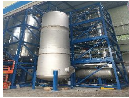
2) Distillation for radiopurity
