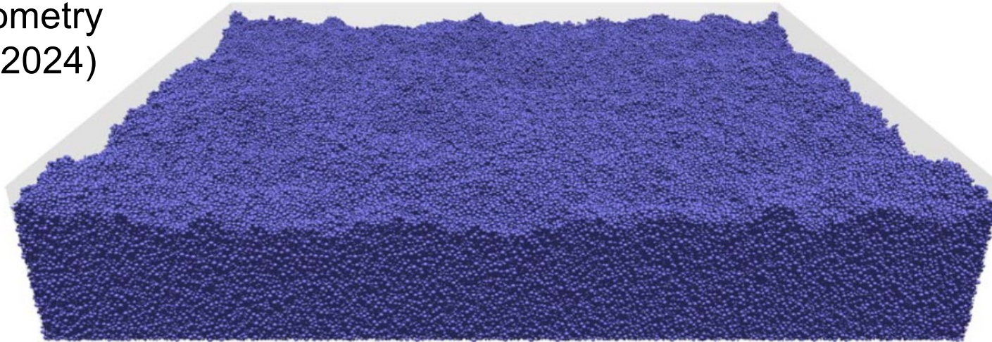
Figure 7. Example realization of a surface with the geometry parameters having the median values from the MCMC samples. The Hurst exponent has a value of H = 0.606 and the surface amplitude \sigma = 0.0998 . Packing density \nu is approximately 0.55, and the particles are as in Figure 4.
