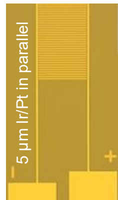
Transition of 5 \mu\text{m} wide Ir/Pt stripes
