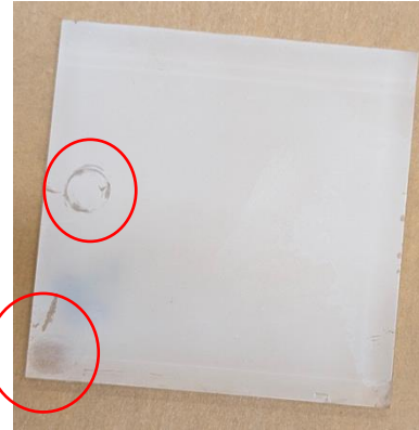
UVT acrylic sprayed with acetone + pTP
